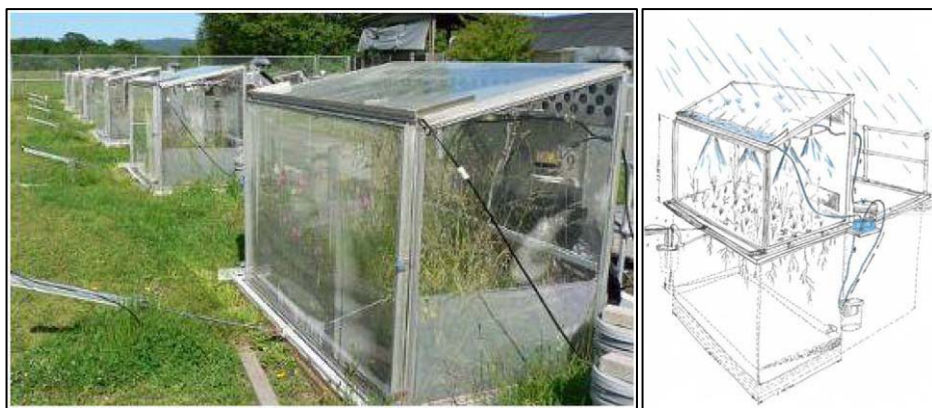
Figure 2. A photograph of the terracosms in an open field in Corvallis, Oregon, and a drawing illustrating the enclosed aboveground chamber, underlying lysimeter, and irrigation system. Additional photographs and diagrams can be viewed at www.teraglobalchange.org .
